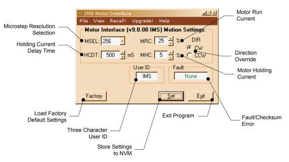
Figure 2.6.7: SPI Motor Interface Motion Settings Screen
